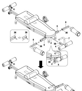
Turn the frames (6) by 90° and insert back into the frames (5).
