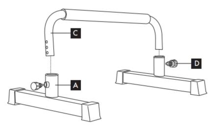
To adjust the height, unscrew the hand knob (D) and adjust the height. Always adjust the height evenly.
