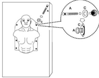
Insert dowels with washers into the holes.
