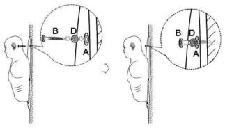
Insert the rubber washers into the screw and insert the screws into the dowels.
