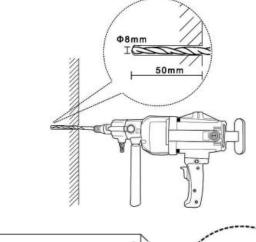
Drill 6x holes with a diameter of 8 mm and a length of 50 mm.
