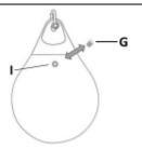
Unscrew the plug (G) using a screwdriver.
