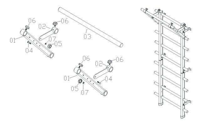
Connect the frames (1 and 2) using the bolts (4), washer (7) and nut (5). Make sure both frames are symmetrical, the arrows must be pointing up. Then push the handle (3) through the frames. Then hang the crossbar on the wall bars and secure with the hand knobs (6).
