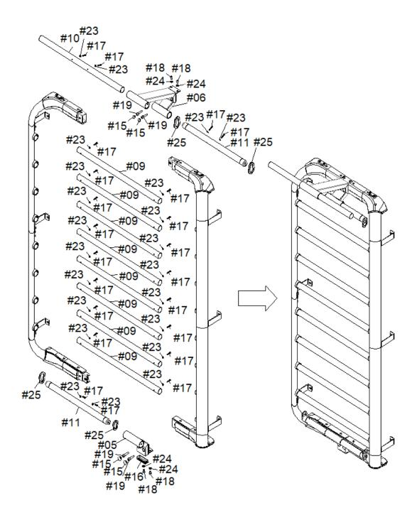
Attach the bar (11) to the step holder (05) using screws (17), washers (23) and cover (16).
