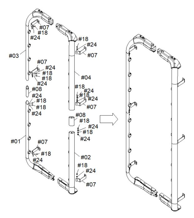
Attach the connecting frame (08) to the lower frame (01) using screws (18), washers (24) and a wrench (28).
