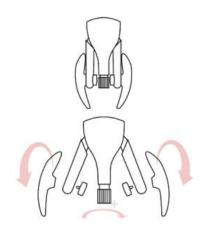
You can adjust the position of the supports using the hand knobs. Always adjust the position symmetrically.
