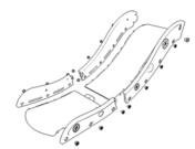
2. Install the slideway handrail
