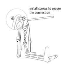
1. Install load-bearing rod and bottom base
