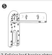
2. Splicing load-bearing plates and backboards, install nut.
