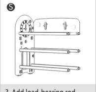
3. Add load-bearing rod, install with nut.
