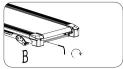
Over time, the running belt (20) will loosen. To tighten the belt, turn both the left & right-side adjustment bolts one full turn clockwise. Check the tension of the belt. Continue this process until belt is at the correct tension. Make sure to adjust both sides equally to ensure even belt alignment. Refer to image C.
