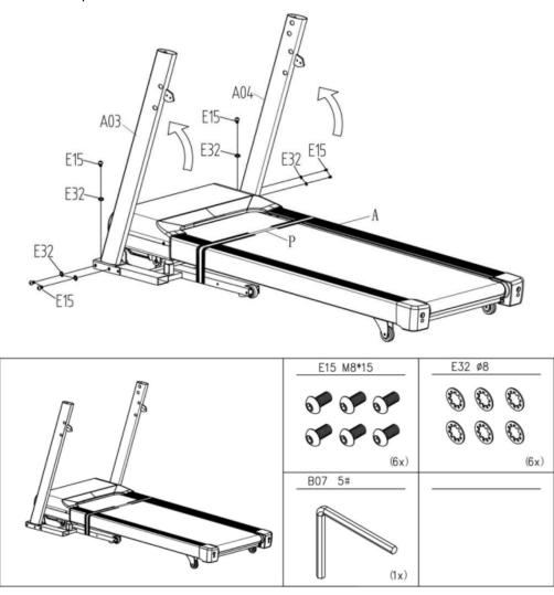
**Step 3**Attach the control panel to the attached posts. On the right side, connect the cables.
