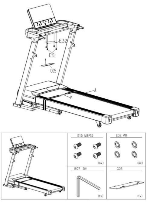
**Step 6**Attach the handles to the posts and control panel.
