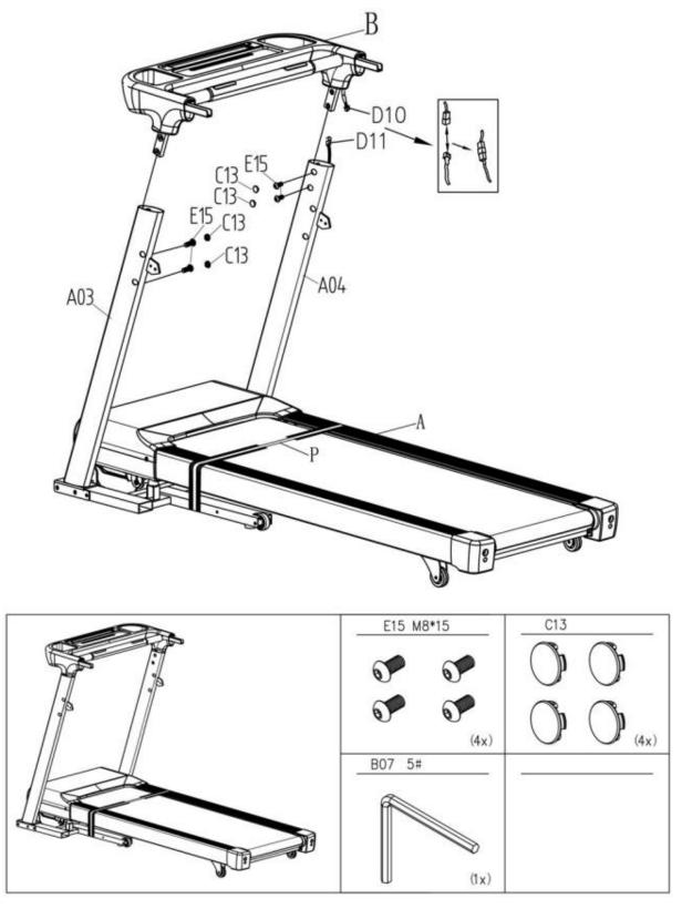
**Step 4**Connect the control panel and display cables. Attach the display to the control panel.
