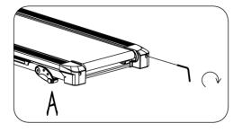
If the running belt (20) drifts to the left, turn the adjusting bolt on the left side ¼ of a turn clockwise, then turn the right adjustment bolt ¼ turn counter-clockwise. If the belt does not move, repeat this step until it centers. Refer to image B.
