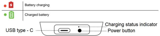
The insoles are powered by 2000 mAh / 3.7 V batteries. To start, press the power button on the
