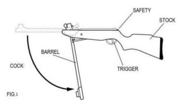
**Warning**: Hold the barrel firmly during cocking so that it does not suddenly spring back and cause injury. Be careful when breaking and keep your fingers away from moving parts of the mechanism. (Fig. 2)
